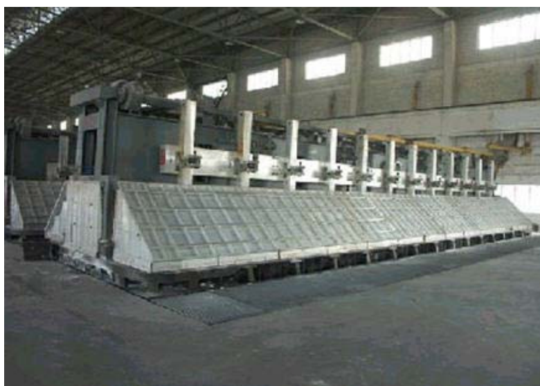
Figure 3-17: Electrolytic Cell for 300 kA Prebaked Carbon Anode Technology in the Cell Room
