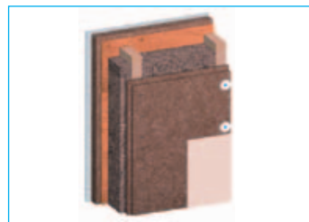
Exterior Insulation and Finishing System (EIFS)
