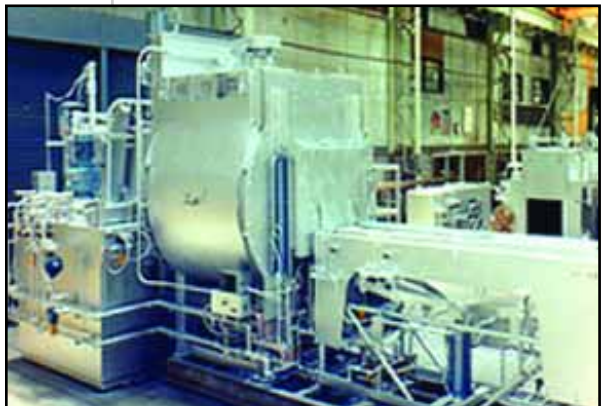
Fig 12: Oil Quenching System, courtesy of Hoeganaes Corp
